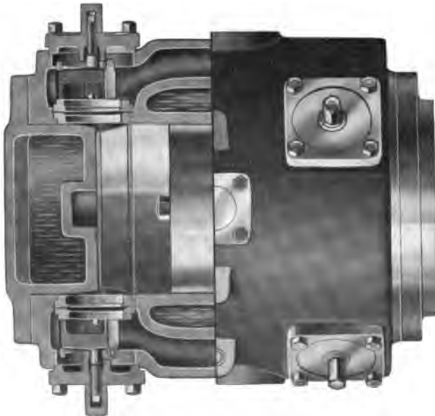
FIG. 61.—Laidlaw-Dunn-Gordon Air Cylinder, with Valves in Place.
