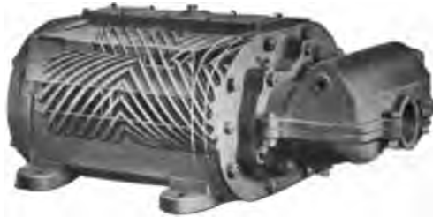
FIG. 191.—Compressed-Air Turbine for Longwall Coal Cutter, Jeffrey Mfg. Co.
