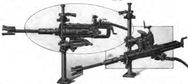
FIG. 205.—Sullivan "Post Puncher." At the left, the machine is arranged for breastwork or undercutting; at the right, for shearing.
